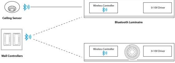
**Bluetooth Luminaire with Integral Sensor**
